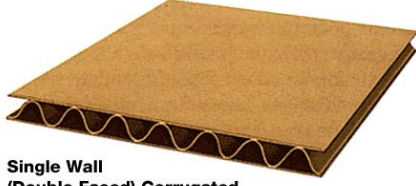
Single Wall (Double Faced) Corrugated
